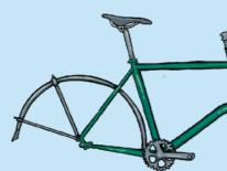
Attach the two V-stays to the rear mudguard using the provided nuts and bolts. Mount the rear mudguards on the bike using the black T25 torx for the V-stays, and the bolts and washers provided in the bag to fasten the mudguards to the rear triangle.
