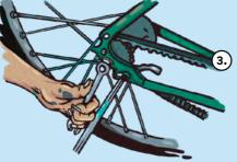
When mounting the rear wheel, make sure to have the sliding inserts loose which makes it easier to fit the belt on the front and rear sprocket. Remember the fixing washer and make sure the gear arm on the hub is pointing forward. Then tighten the nuts to 30-45Nm with your 15mm wrench,
