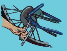
3. When mounting the rear wheel, make sure to have the sliding inserts loose which makes it easier to fit the belt on the front and rear sprocket. Remember the fixing washer and make sure the gear arm on the hub is pointing forward. Then tighten the nuts to 30-45Nm with your 15mm wrench.
