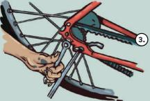
make sure to have the sliding inserts loose which makes it easier to fit the belt on the front and rear sprocket. Remember the fixing washer and make sure the gear arm on the hub is pointing forward. Then tighten the nuts to 30-45Nm with your 15mm wrench
