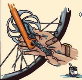
2. Remove the protective plastic inserts from the brake calipers. Mount the front wheel first, and make sure to grease the thru axle. Tighten the axle to 10 Nm maximum using a 6mm allen key.
