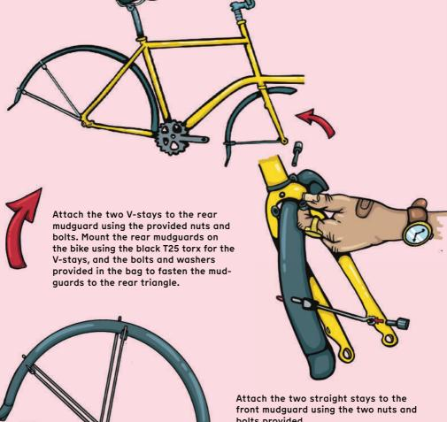
Don't forget to take out the wheels before you install the mudguards. Oritjust ain't happening! Once installed, put the Wheels back on to adjust the Mudguards.
