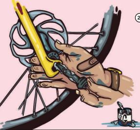
2.) Remove the protective plastic inserts from the brake calipers. Mount the front wheel first, and make sure to grease the thru axle. Tighten the axle to 10 Nm maximum using a 6mm allen key.
