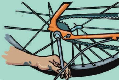
4. Tighten the belt. The easiest way to do this is by using the 15mm wrench and applying pressure on the right hand side nut, which moves the wheel and the sliding inserts back. When the inserts are back and the belt is tight you tighten the inserts with your 6mm allen key.
