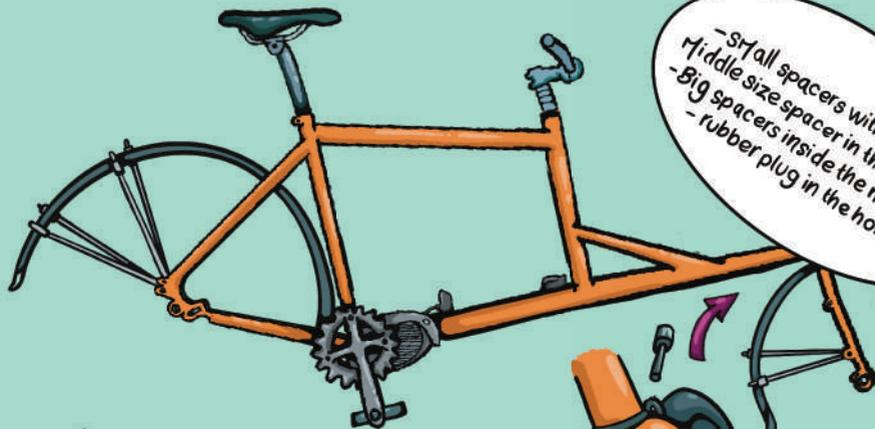
Attach the two V-stays to the rear mudguard using the provided nuts and bolts. Mount the rear mudguards on the bike using the black T25 torx for the V-stays, and the bolts and washers provided in the bag to fasten the mudguards to the rear triangle.
