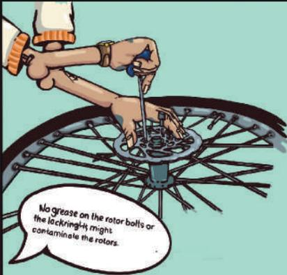
1. Mount the provided 160mm 6 bolt rotor on the front wheel using the 6 torx-25 rotorbolts. Tighten the opposite bolts in star pattern. Tighten them to 6,2Nm. Look out for the arrows on the rotors, to make sure they are mounted correctly.
