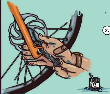
2. Remove the protective plastic inserts from the brake calipers. Mount the front wheel first, and make sure to grease the thru axle. Tighten the axle to 10 Nm maximum using a 6mm allen key.
