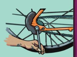
(3.) When mounting the rear wheel, make sure to have the sliding inserts loose which makes it easier to fit the belt on the front and rear sprocket. Remember the fixing washer and make sure the gear arm on the hub is pointing forward. Then tighten the nuts to 30-45Nm with your 15mm wrench.
